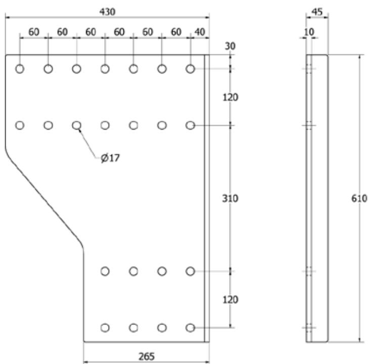
Install the coupling head about 300 mm below the frame with these side plates.
