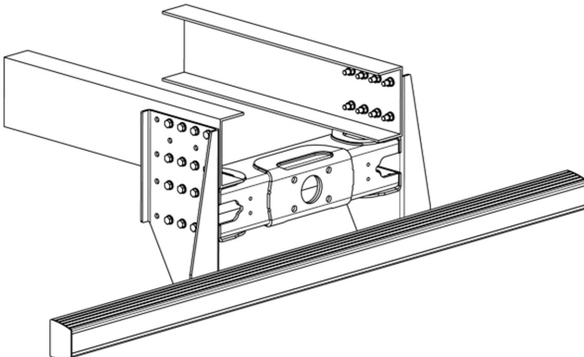
Install the underrun protection on the TAV702 side plates or, with separate fasteners, on the vehicle's frame.
