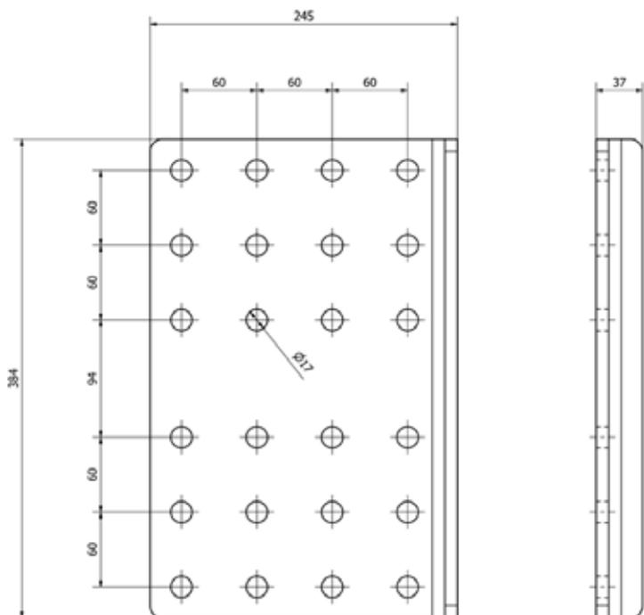
Install the coupling about 100 mm below the lower surface of the vehicle's frame with these side plates.
