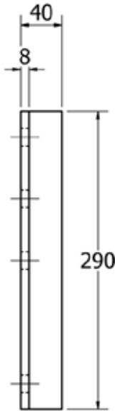
Use these side plates to install the coupling head at the height of the frame beam lower surface. Install the side plate with the strengthener bent forward. Delivered in pairs.
