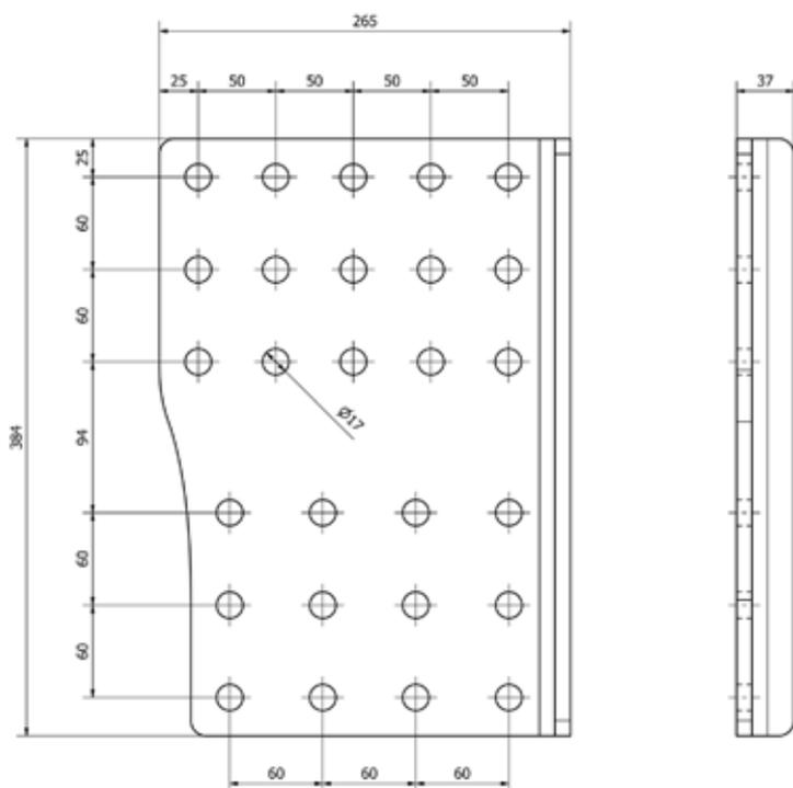
Install the coupling about 100 mm below the lower surface of the vehicle's frame with these side plates.
