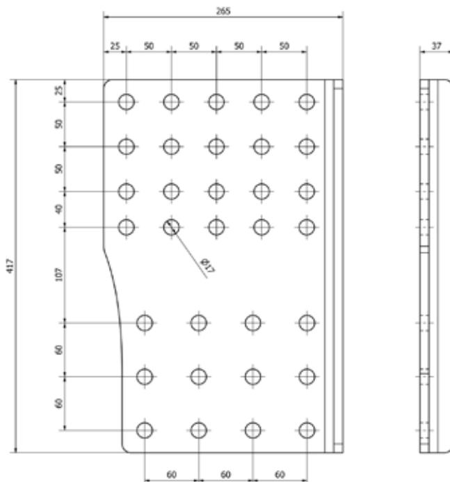
Install the coupling about 100 mm below the lower surface of the vehicle's frame with these side plates.
