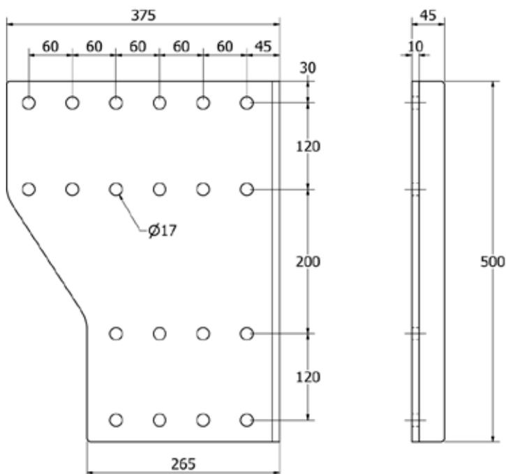
Install the coupling head about 200 mm below the frame with these side plates.
