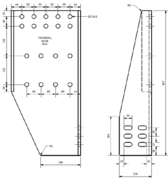
Use these side plates to install the coupling at the same height of the frame beam lower surface.
