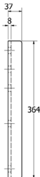
Install the coupling head about 100 mm below the lower surface of the vehicle's frame with these side plates. The side bars can be used to move the drawbeam forward by about 50 mm. Delivered in pairs.
