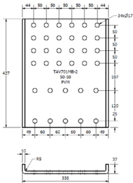
Install the coupling about 100 mm below the lower surface of the vehicles' frame with these side plates.
