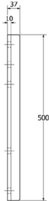
Install the coupling head about 200 mm below the frame with these side plates.
