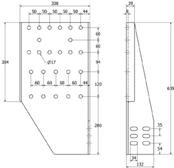
Both the drawbeam and the underrun protection can be installed on the side plates.
