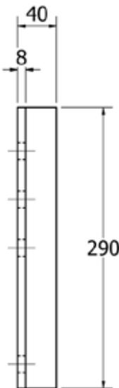
Use these side plates to install the coupling head at the height of the frame beam lower surface. Install the side plate with the strengthener bent forward. Delivered in pairs.
