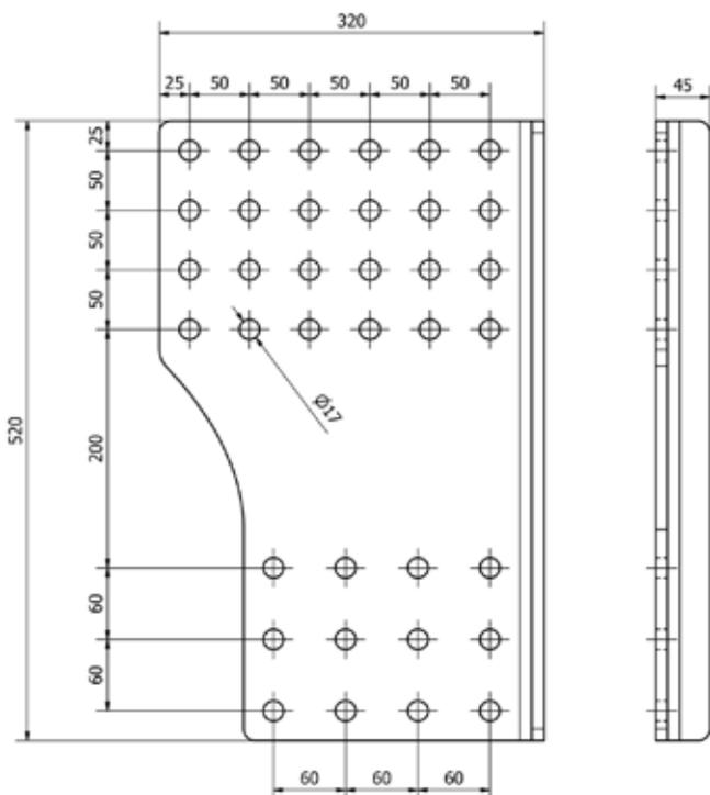
Install the coupling head about 200 mm below the frame with these side plates.
