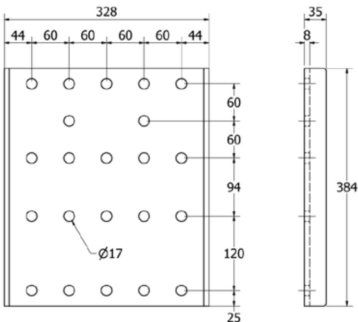
Install the coupling head about 100 mm below the lower surface of the vehicle's frame with these side plates. The side bars can be used to move the drawbeam forward by about 60 mm. Delivered in pairs.
