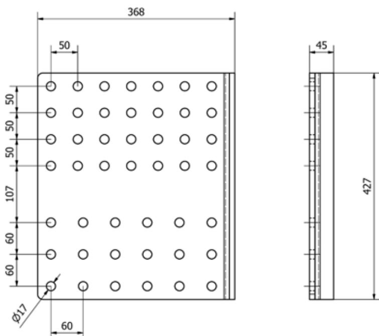
Install the coupling about 100 mm below the lower surface of the vehicle's frame with these side plates.
