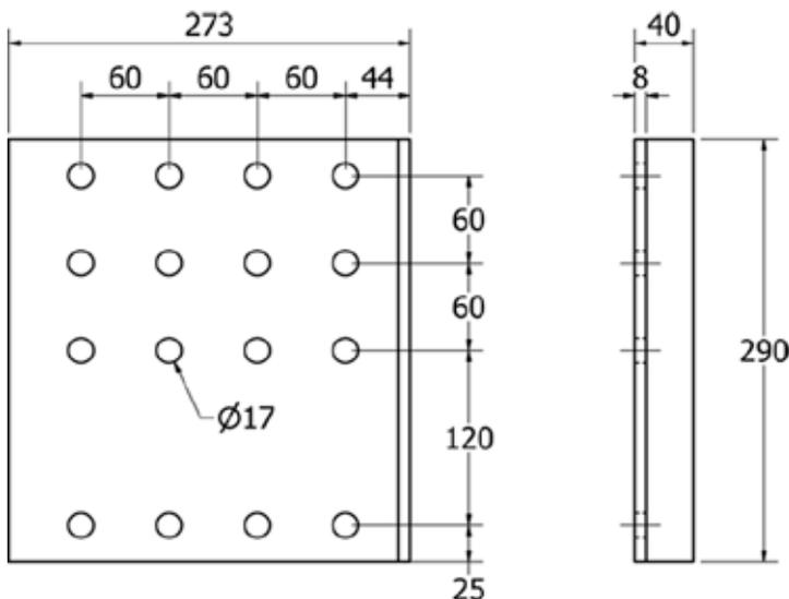
Use these side plates to install the coupling head at the height of the frame beam lower surface. Install the side plate with the strengthener bent forward. Delivered in pairs.
