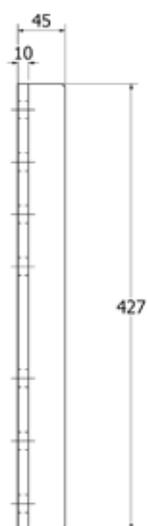
Install the coupling head about 100 mm below the lower surface of the vehicle's frame with these side plates.
