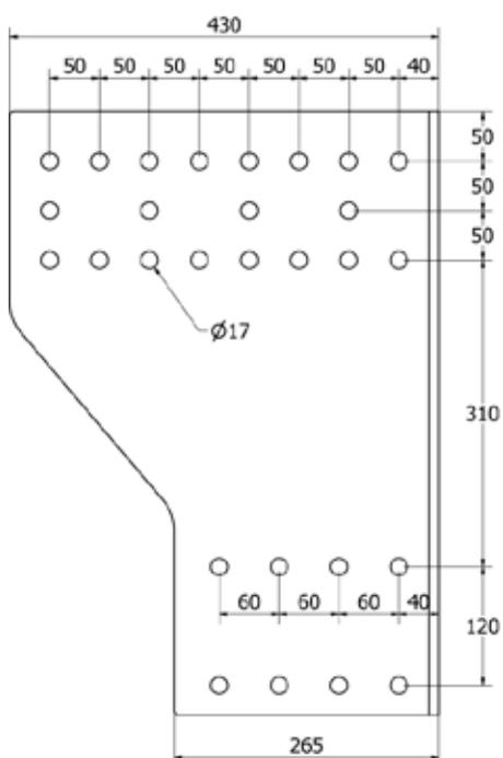
Install the coupling head about 300 mm below the frame with these side plates.
